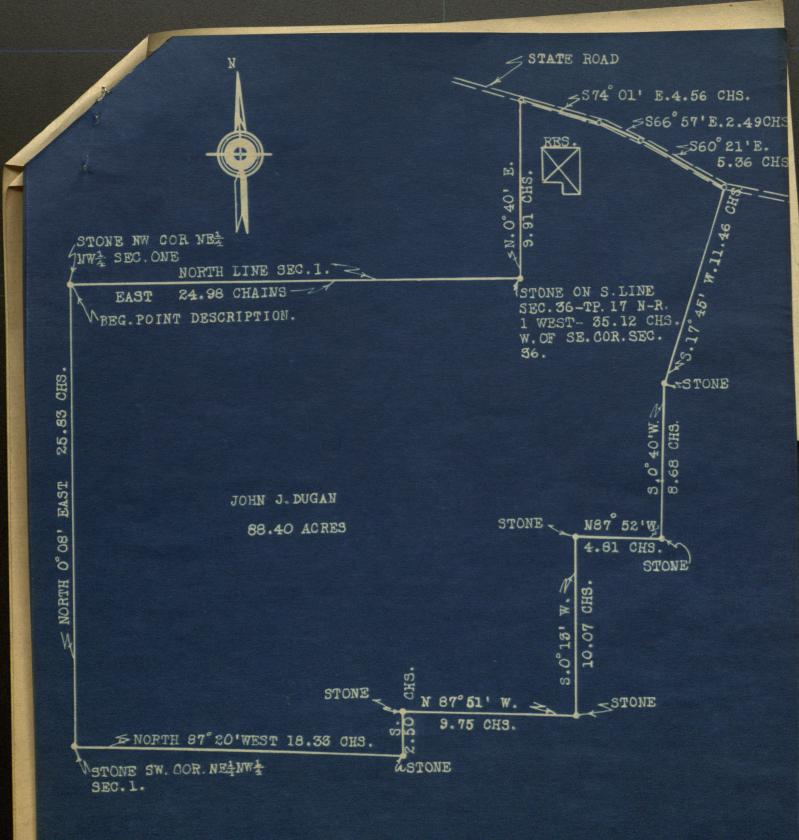
SURVEY FOR JOHN J.DUGAN OF A PART OF THE NE<sup>1</sup>/<sub>4</sub> OF THE NW<sup>1</sup>/<sub>4</sub> OF THE NE<sup>1</sup>/<sub>4</sub> OF FRACTIONAL SECTION 1, TOWNSHIP 16 NORTH OF RANGE 1, WEST, AND A PART OF THE SW<sup>1</sup>/<sub>4</sub> OF THE SE<sup>1</sup>/<sub>4</sub> OF SECTION 36, TOWNSHIP 17, NORTH OF RANGE 1 WEST.ALL IN HENDRICKS COUNTY, INDIANA.
